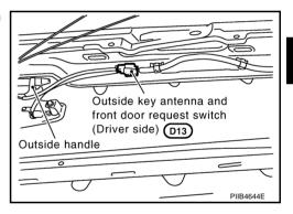
9. Remove the outside handle mounting bolts, move the outside handle assembly backward, and then remove it from the panel in front of the outside handle escutcheon.
