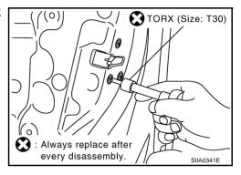
5. Remove the outside handle mounting bolts, and move the handle backward to disengage it from the panel in front of the outside handle escutcheon, then remove the handle.
