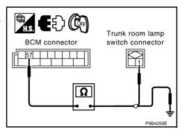
3. Check continuity between harness connector B4 terminals 57 and ground.
