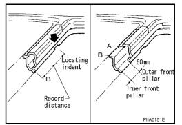
Prepare a cutting jig to make outer pillar easier to cut. Also, this will permit service part to be accurately cut at joint position.
