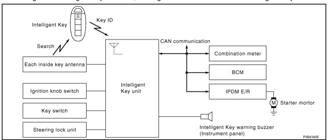
When ignition knob switch is ON (press ignition switch), Intelligent Key unit searches Intelligent Key in the vehicle using inside key antenna.
