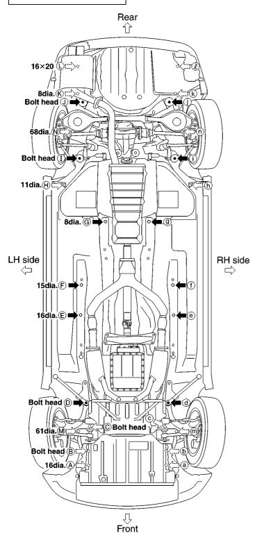
Coordinates: (A),(a) ①,(i) X:413 X:473 Y:-368 Y:2604 Z:305 Z:114 (B),(b) (J),(j) X:411 X:452 Y:-261 Y:3164 Z:95 Z:179 (C),(C) (K)X:395 X:550 Y:76 Y:3265 Z:120 Z:316 (D),(d) (k) X:388 X:-500 Y:279 Y:3273 Z:47 Z:316 E,@ €,@ X:438 X:535 Y:1100 Y:3540 Z:79 Z:329 **(F)**,**(f)** X:440 Y:1400 Z:79 **G**,**9** X:205 Y:1992 Z:59 (H),(h)X:605
