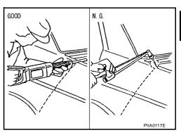
• When welding HSS panels, use spot welding whenever possible in order to minimize weakening surrounding areas due to
