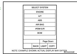
Select diagnosis mode. "WORK SUPPORT", "SELF-DIAG RESULTS", "CAN DIAG SUPPORT MNTR", "DATA MONITOR", "ACTIVE TEST" and "ECU PART NUMBER" are available.
