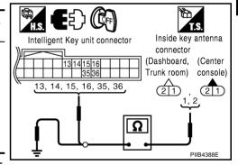
Check continuity between inside key antenna harness connector M172 (center console), M69 (dashboard), B114 (trunk room) terminals 1, 2 and ground.
